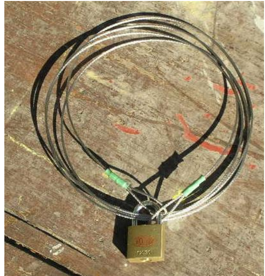
Padlock through eyelets and around tether coils.
